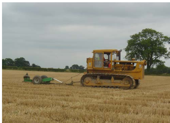
Figure 30. Installing mole drains
