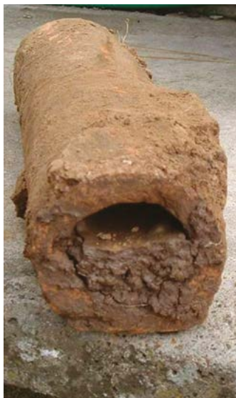
Figure 22. Silted clay drain
