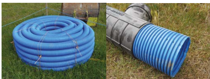
Figure 36. Modern perforated plastic drainage pipe
